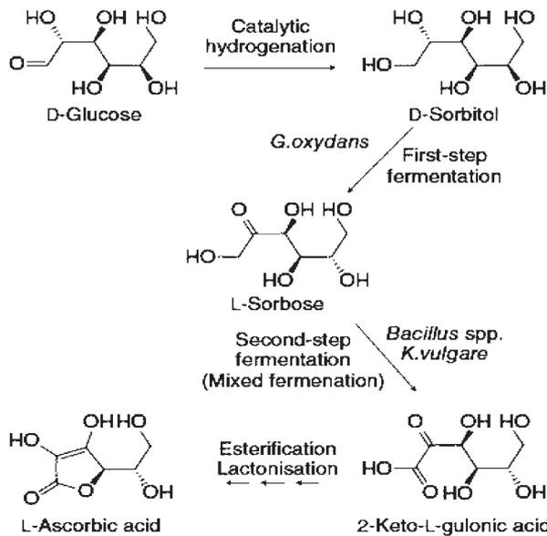
Fig. 5 Current method for industrial production of Vitamin C (fig adopted from Ref. 5)
